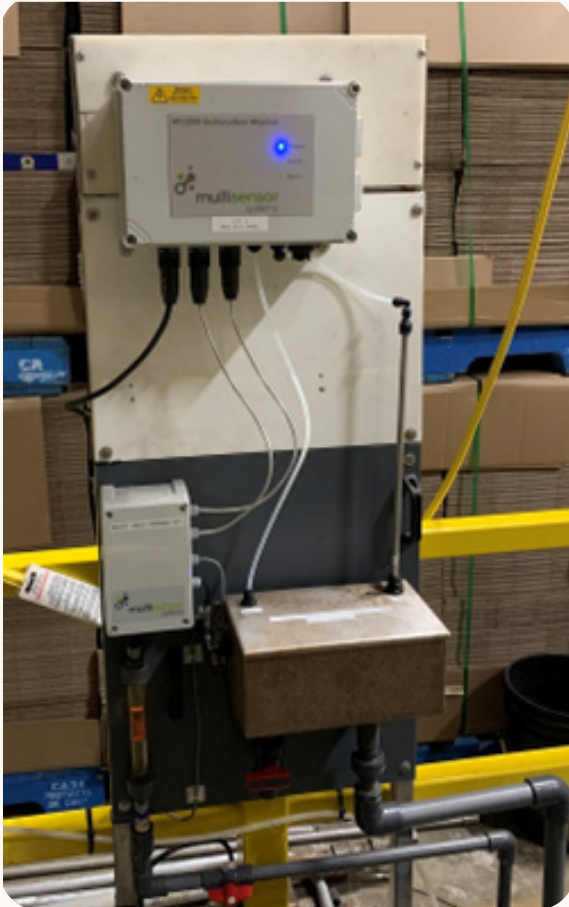
The MS1900 analyser installed close to the effluent.
